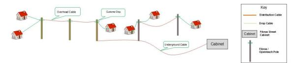
The majority of installation will be overhead, however in some cases we also use a combination of Fibrus and Openreach underground duct or simply the Openreach underground duct.
