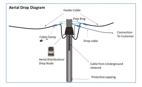
The feeder cables are then used to distribute the fibre to customers along the pole route. Feeder cables are passed through the distribution points while individual customer drops are made available for customer connections. The capacity of the 48 fibre can be maximised with the strategic placement of splitters within specific distribution nodes.
